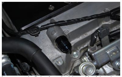
12. You now need to remove the fitting from the drivers side of the valve cover, this is done easily with a pair of channel locks or pliers, rock this back and forth applying outward pressure until the fitting comes out.
