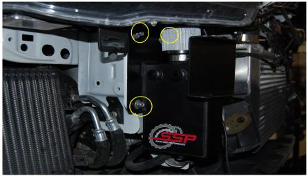
9. The can is installed using the same 4 – 12mm bolts that held the OEM bracket in (see above picture). If you purchased our matching driver's side lightweight bumper bracket, you can go ahead and install this as well.
