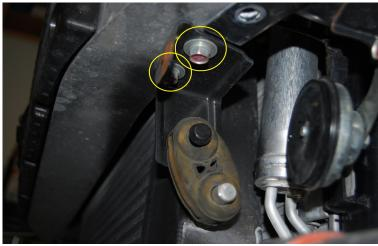
6. On each end of the crash beam where you removed the foam pads, you will find 4 holes, in them are 12mm bolts holding the beam to the brackets, remove those (these will not be reinstalled on the new brackets or catch can) as well as the 2 bolts on the top and bottom of the beam that mount it to the bracket.
