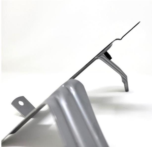
Step 3: Assemble the ECU to the honeycomb mounting plate using the right had side 16mm length bolts and lock nuts. Next install the top left 20mm bolt into the ecu plate, going through the ecu and securing into the logo plate. The bottom left mounting hole will REMAIN OPEN for now. **\*\*NOTE: Picture does not show an ecu installed here, however it should be installed on the bracket at this time\*\***
