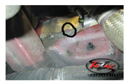
2. Bend or remove this stud, easily done with a small hammer. This stud will rub the dump tube and cause noises inside the car. Try to get it flat on the firewall (as shown below) or completely remove it.
