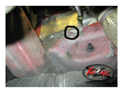
3. Install the dump tube and waste gate as shown. Make sure the tube does not touch the AC line nor the firewall. Orient the outlet of the dump from under the car, making sure it is pointing directly to the ground. Keep it from pointing at the axle or transfer case, it may take adjustment of the wastegate as well as dump tube to line this up correctly.
