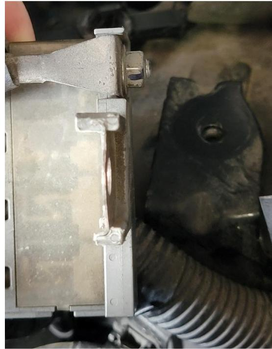
**Step 5:** Prepare the tray assemblies by installing the stick on foam strips as shown.
