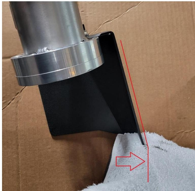
**Step 4:** Install intake assembly and heat shield. Heatshield is mounted with long allen bolt and fender washer through the shield and supported by the included long spacer. **\*\*START THIS BOLT CAREFULLY AND STRAIGHT**, it is easy to damage the thread since it is so long\*\*
