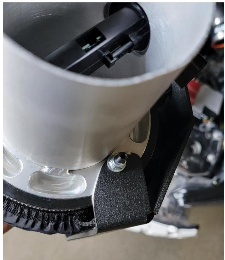
**Step 3:** ETS Heatshield Modification 2 – Drill out lower mounting hole to 23/64" or 3/8". Bend lower mounting ear back to a LESSER bend as shown. This may need to be tweaked for fitment.
