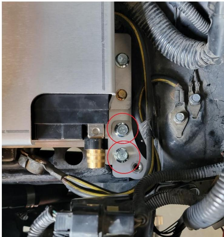
**Step 2:** ETS Heatshield Modification 1 – Mark and drill new mounting ear hold 1" down from current position. Cut down and reshape end of bracket
