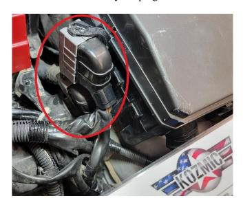
**Step 2:** Remove the **SMALL** ECU Connector Shroud by lightly pushing in on the 4 lock tabs as seen in the picture. If the shroud has tape at the end around the harness, remove this tape before attempting to remove the shroud to make it easier.
