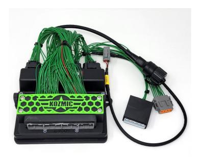
Step 8: The main ECU bracket is now assembled and ready to install. Any sub wiring, CAN wiring etc should be performed now or once installed in the car. Reinstall the ECU assembly into the car. This is a tight fit! Watch the patch harness wiring on install and once installed for rubbing on sharp edges.
