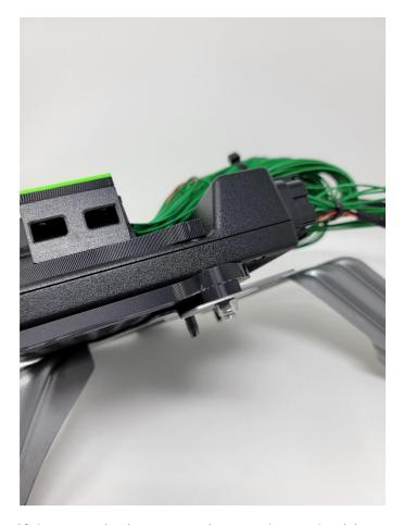
Step 5: Plug the patch harness into the ECU. At this time if there are zip ties or coverings on the patch wiring itself this is a good time to remove them to allow the wire to rotate and flex as needed. Route the OEM connector assembly over the ECU bracket and into the holder mount. Install the securing logo plate with the supplied 16mm bolts.
