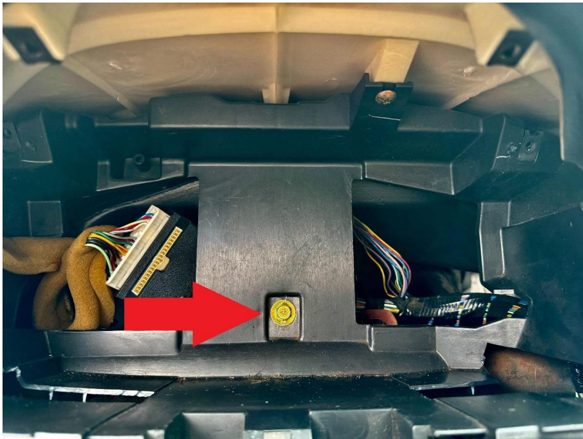
**Step 11:** Connect the 2 factory harness plugs into the adapter box carefully. They should be a firm but easy fit into the housing, do not force them if they do not want to go in, instead remove and assure there are no bent pins.
