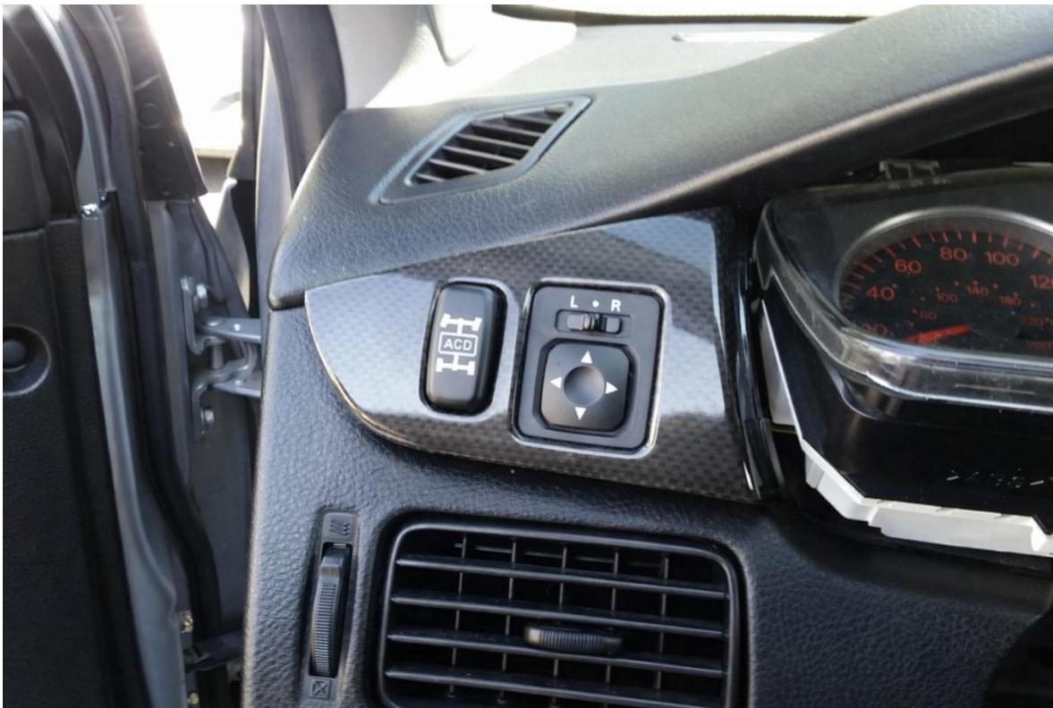
**Step 7:** Now you will have clearance to rotate the OEM cluster to unplug the 2 connectors in the top corners. Once unplugged, carefully rotate and remove the cluster from the dashboard.
