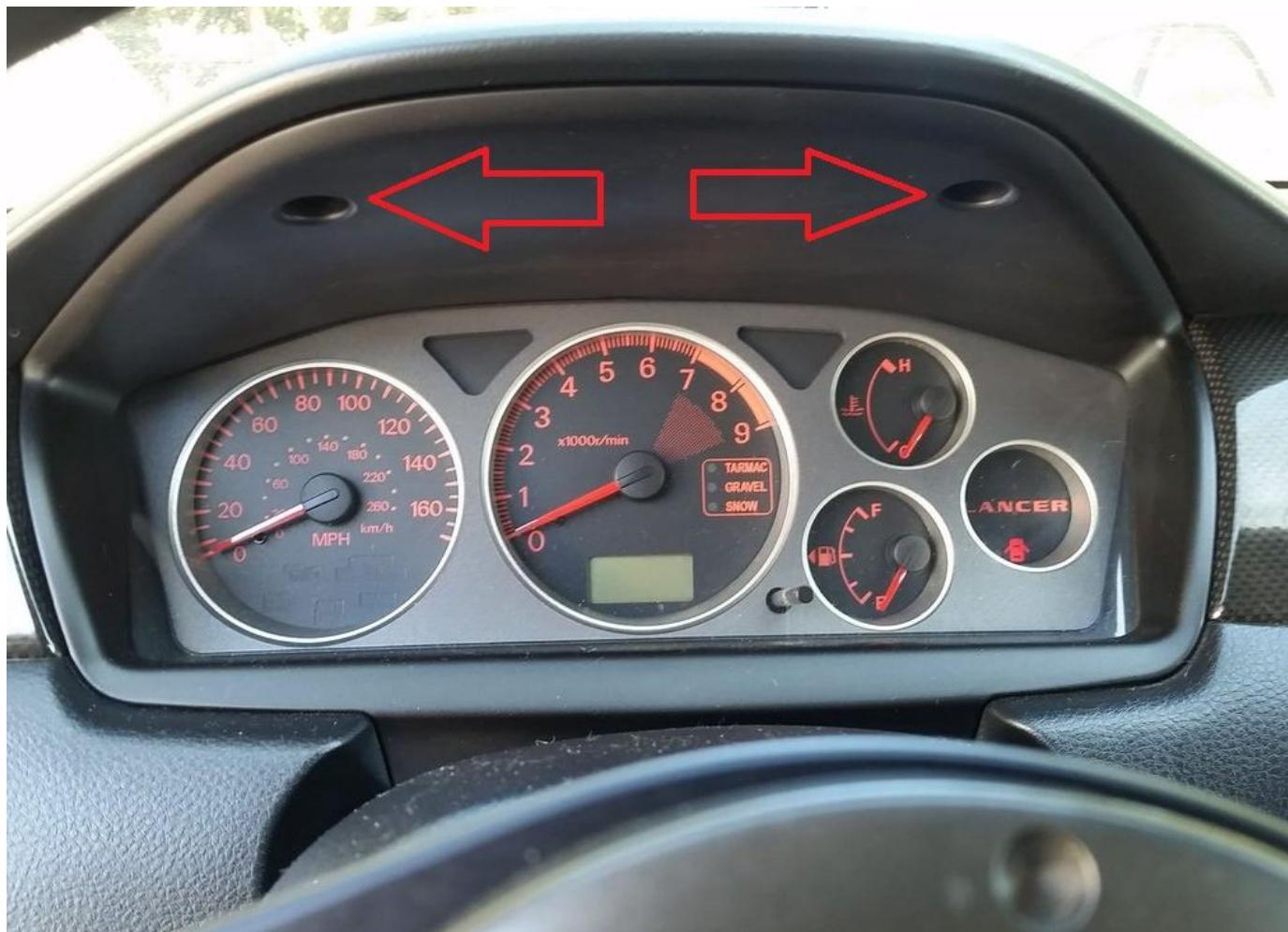
**Step 5:** Remove the 3 screws securing the factory gauge cluster – **Do not discard as these will be used to mount the new bezel assembly.**
