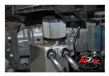
Step 4: Route hoses. There are 2 hoses, they will need to be cut to length. The first hose will go on the PCV hose routing back to the intake. You need to remove the OEM hose, attach the new hose to the valve cover. If you are still routing the oem hose back into your intake, you will need to cap off your intake breather port.
