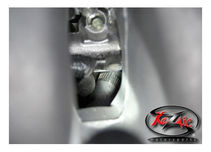
Make sure that when you are routing the hoses to the catch can, they are secured out of the way of anything that might rub or tear them. The hoses will simply push onto the pushlock fittings provided, no clamps needed.
