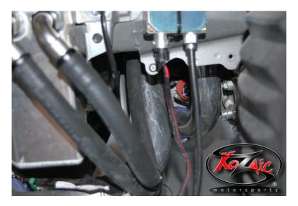
Step 5: Make sure the filter and Allen drain plug are secure on the can if not already. We recommend using thread sealant tape on the threads of the drain plug to assure no small leaks in the can – <u>Drain Plug TQ: 120 in/lbs.</u> Drain intervals will depend on HP level and health of the engine. We recommend draining the can on your first oil change and determine the drain interval based on amount you find on your first drain.
