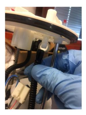
**Step 3:** Disconnect electrical plugs on fuel hat. Compress basket and remove snap ring on side post. The basket will now come part and give you access to remove the fuel pump. Unclip the fuel pump and remove from the basket. Using a flat blade screw driver remove the electrical harness and the pump mounting ring.
